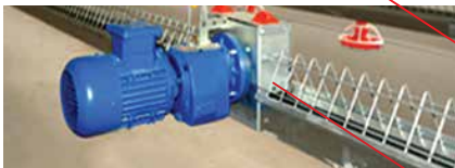
Drive unit for suspended chain feeding system
